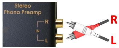
If no change, return the input cables to their proper jacks and then proceed next to swap the left and right plugs at the preamp's OUTPUT. If the problem now switches speakers, the preamp is most likely at fault. If no change, check the output cable and amp/receiver for a problem.
